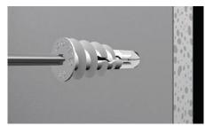
Press tip of SnapSkru anchor into drywall using PZ2 or Phillips #2 screwdriver or screw gun. Drive the anchor clockwise into drywall until anchor stops flush with the outer wall surface.
